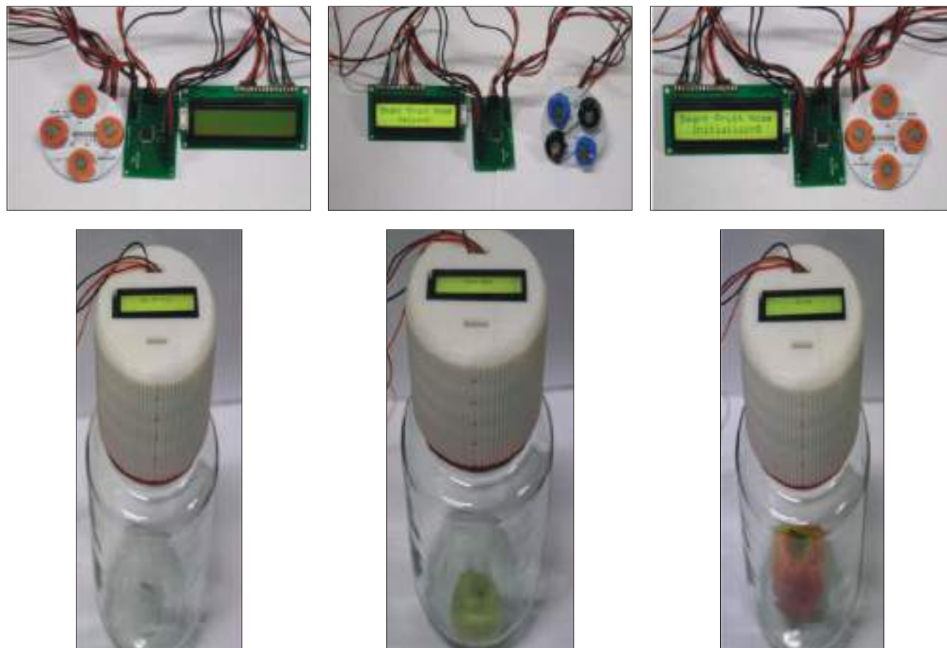
E-Nose for apple – Prototype developed by IIT, Roorkee and evaluated for apple maturity indices and quality analysis
