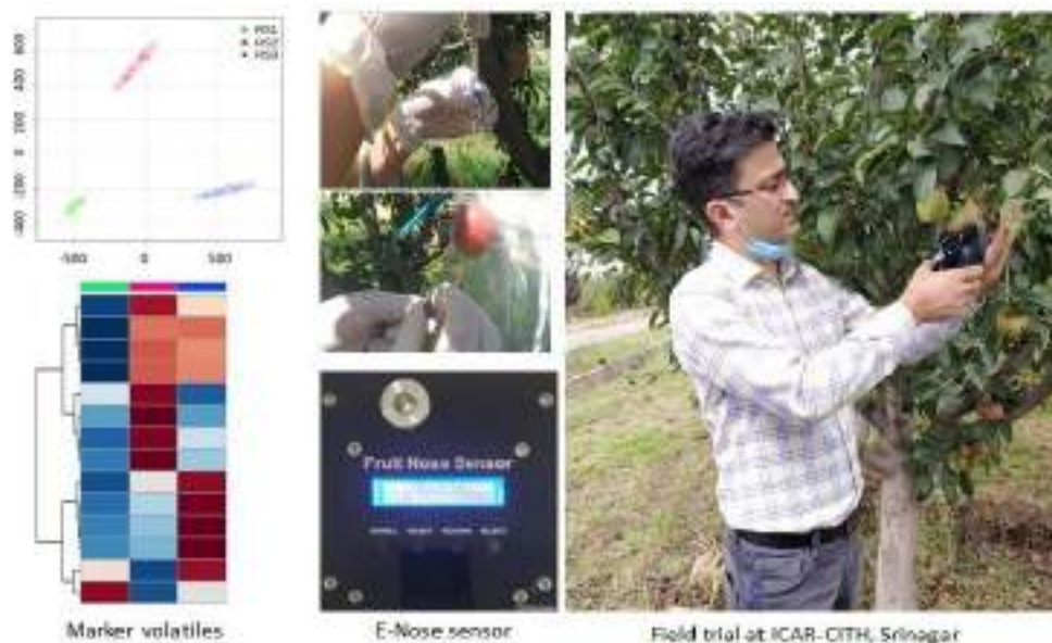
Fig-20: E-nose for non-destructive determination of ripening and quality attributes of apple
