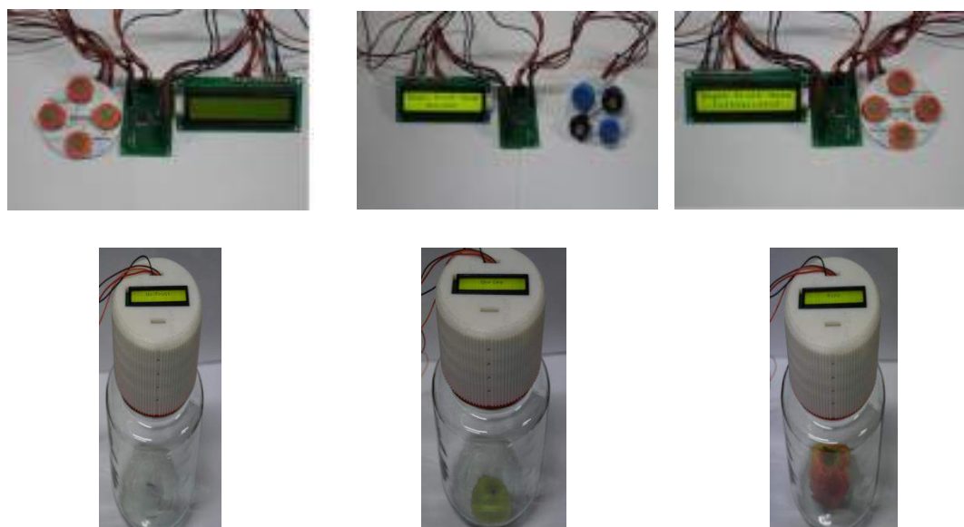
E-Nose for apple – Prototype developed by IIT, Roorkee and evaluated for apple maturity indices and quality analysis
